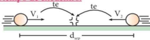
$$t_e = \frac{d_{sep}}{V_1 + V_2}$$
